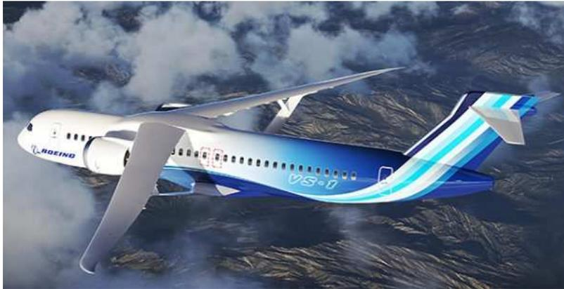
In the meantime, **NASA is partnering with the U.S. aircraft manufacturer to fly a "full-scale" demonstrator of a high-stretch, high-stay wing aircraft by 2028**, with the TTBW configuration theoretically able to reduce fuel consumption and emissions by up to 30 percent compared to the latest generations of current single-aisle aircraft, also capitalizing on ongoing advances in propulsion, materials and systems architecture.
