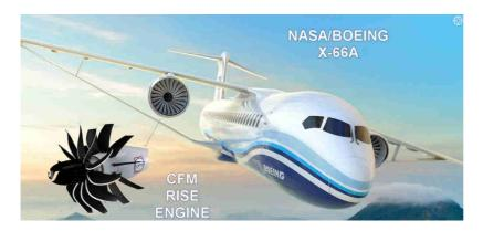
In the infographic above, provided by Boeing, the wings are mounted above the fuselage.
